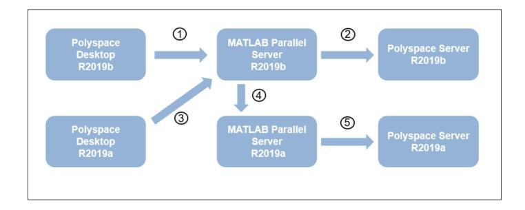
To support submissions from multiple releases with a single MATLAB Parallel Server cluster, you have to link the various installations of Polyspace products and MATLAB Parallel Server. Of the links shown in the preceding figure, the links numbered 1, 2 and 5 are part of a regular server-client installation using all products from the same release. To create all the links, do these steps:
